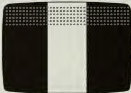
The picture is actually composed of 525 adjacent lines, which are scanned from left to right, beginning with the top line and ending with the bottom line.
