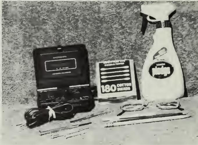
Basic film equipment restoration kit, including everything but lens tissue: small screwdrivers, fine point tweezers, pencil and ballpoint erasers, emery board, close-up glasses, volt and current meter, film path swabs, and wax.
