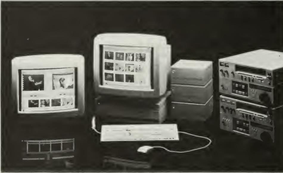
A complete Avid desktop video system includes (left to right): two Macintosh monitors (record and playback), a mouse and keyboard, a central processing unit, three hard disk storage modules, and two video decks.
