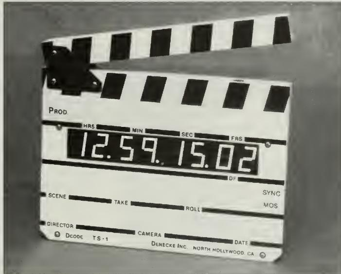
SMPTE time code is the glue that holds the video world together. It is a complex sync reference that can lock one video machine to another or to many others, or a video recorder to a multi-track audio recorder. Its most important characteristic is that it keeps track of time as a series of continuously generated numbers. These numbers allow the user to locate a particular frame on a videotape—an address—and lock two machines together synchronously at any given address.
