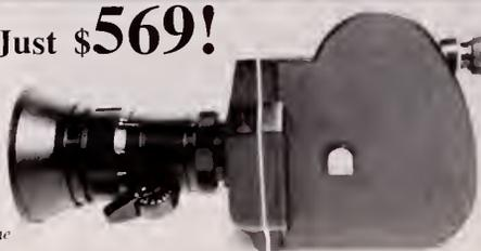
The crystal sync K-3 camera comes with the standard set of accessories (see description at right) and 17-69mm lens. The camera will run at 12, 24, 48fps at sync and with the addition of an Aaton style speed crystal control all speeds between 6 and 60fps are possible. With the addition of the sync motor the K-3 is the ideal camera for music videos, second unit, or stunt camera work, at less than the cost of a traditional crystal sync motor alone. Motor made in USA.
