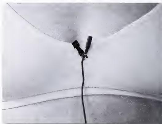
A Sennheiser lavalier clipped to a bra. Whenever mounting a microphone on someone, try to isolate it from the clothing or attach it to the clothing so that it moves easily with, rather than against, the clothing. This clip achieves that purpose but it is rather bulky.
